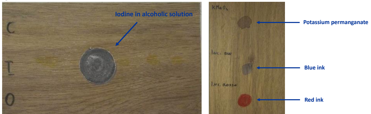
Figure 1: Test for the determination of stain resistance
