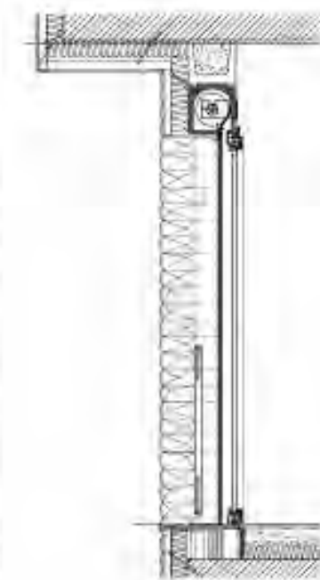
dettaglio verticale B, porta finestra vertical detail B, French door
